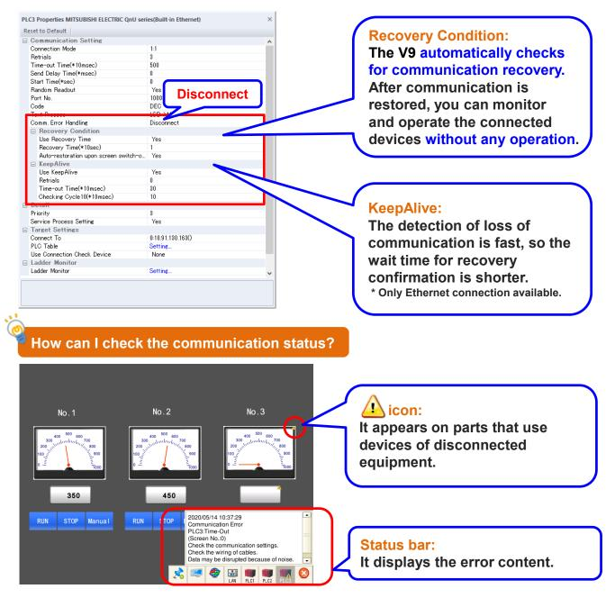
Communication status is also output to system devices \$Px: 00010 or later. You can display the status on a lamp part, for example.
